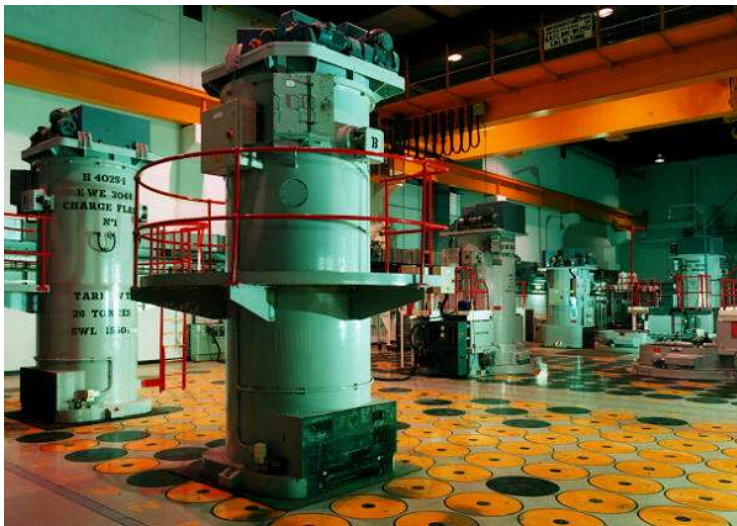
Loading silos with canisters containing vitrified HLW in the UK. Each disc on the floor covers a silo holding ten canisters.
